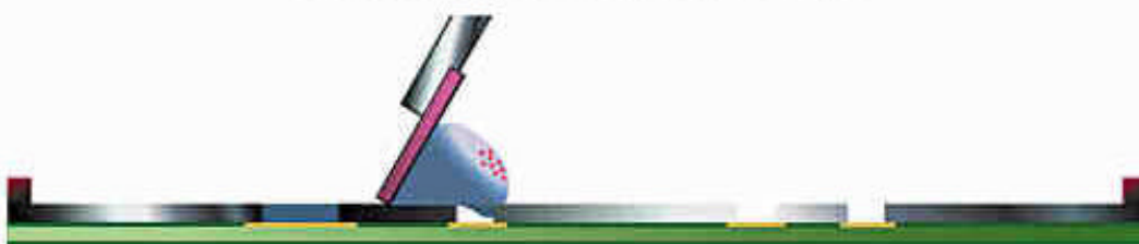
Figure 13. This picture is taken from an animation in PasteMaster®. The animation is based upon a study with high-speed video recordings of aperture filling. It clearly shows the backfill effect when the paste flows into the aperture.
