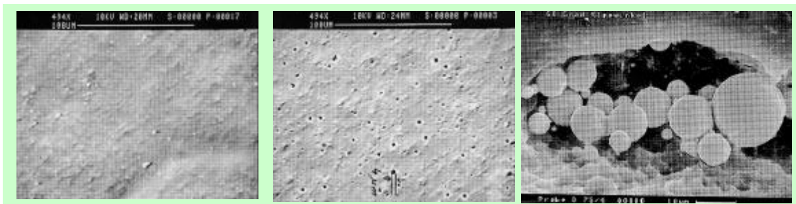
Figure 8: Different solder resists result in different surface morphologies. The picture in the left shows a relatively smooth surface. The surface in the middle picture shows a relatively rough surface with pores up to 4 microns. The right picture shows the edge of a solder resist. These images underline our theory that the solder resist is not a chemically inert, non-porous film. It is capable of soaking up and retaining a substantial amount of process fluids during the board manufacturing process. Pictures courtesy Bell & Zajtischek.
